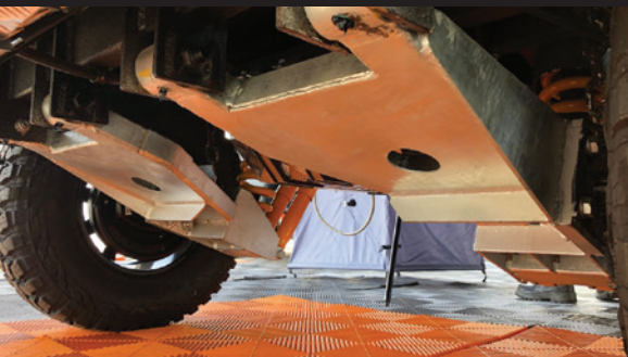
Latest Series 4 Heavy Duty Suspension with Bolt on Stub Axle
